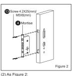
Make the mortise cable get through the door plate, fix the mortise with 4
