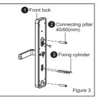
(3) As Figure 3: Install the two connecting pillars with two fixing cylinders onto the front
