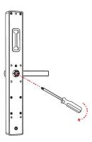
1. Turn the handle on back panel Loosen the inner hexagon screw of the handle counterclockwise
